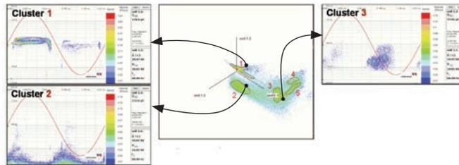
Separation of PD sources by 3CFRD
