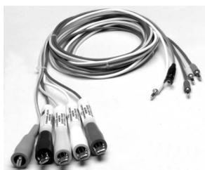
The fused potential leads provides the technician protection when measuring a higher system voltage (600 vac/2 amp fuse).
