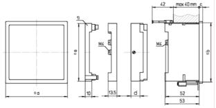
Picture 15: Dimensional drawing EQxx07A and YQxx07A (all dimensions are in mm)
