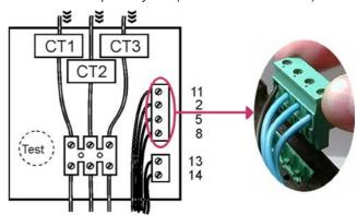
Picture 14:Connections for full equipped device, position of battery and picture of connectors
