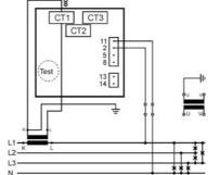
Picture 12:Three phase system (four wire balanced - 4b)
