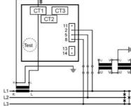
Picture 10:Three phase system (three wire balanced - 3b)
