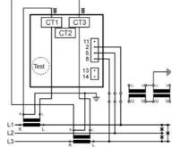
Picture 11 :Three phase system (three wire unbalanced - 3u)
