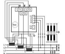
Picture 13:Three phase system (four wire unbalanced - 4u)
